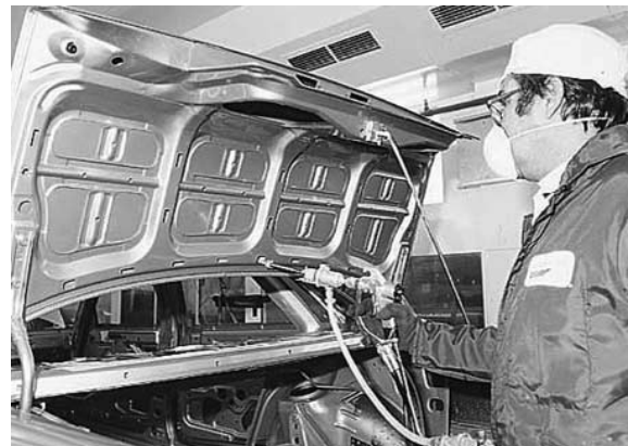
manually dispensed cavity wax
